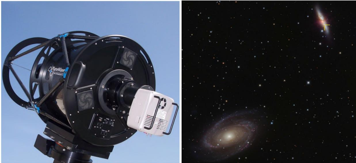
**Figure 1.** The left panel shows the PlaneWave 17-inch diameter mirror telescope proposed here. The right panel shows an image of the galaxy M81 (lower left) and galaxy M82 (top right) and a recent stellar explosion, supernova SN 2014J (yellow crosshair), taken with the same PlaneWave 17-inch telescope (credit: James Morse).
