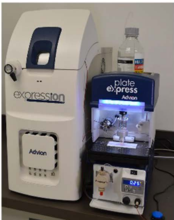
Figure 1 – TLC/MS system used in this work. On the left is the compact mass spectrometer with the PlateExpress extraction device and on the right is the isocratic pump (Advion, Inc., Ithaca, N.Y.). Individual TLC spots were extracted via an extraction solvent delivered from the isocratic pump shown underneath the PlateExpress. The extract from the TLC spot was delivered directly to the ESI or APCI source of the mass spectrometer, which provides a mass spectrum of the TLC spot. Shown here is the Advion expression CMS-L.
